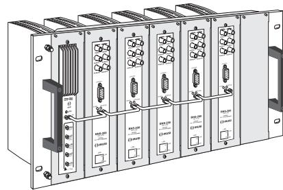
Example of BNS headend. Contains five BNS modules and 1 CFP-900 power supply all fixed on 1 rack-frame SMR-601.
