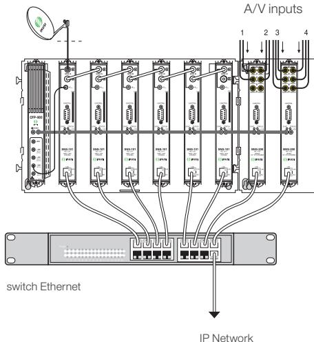
Example of mixed SNS/BNS headend for six digital satellite TV transponders and four video/audio local sources. Contains 6 SNS, 2 BNS-200 and 1 CFP-900 power supply, all fixed on 2 base-plates BAS-700.
